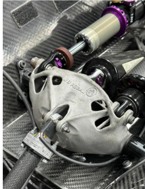
Rocker shafts from 3D Laser BW for the racing car of the Esslingen University of Applied Sciences racing team
